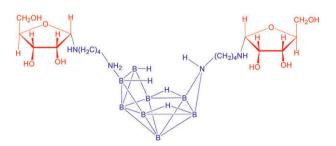
The first synthesis of azanonaborane-containing sugars, possible boron carriers for neutron capture therapy
